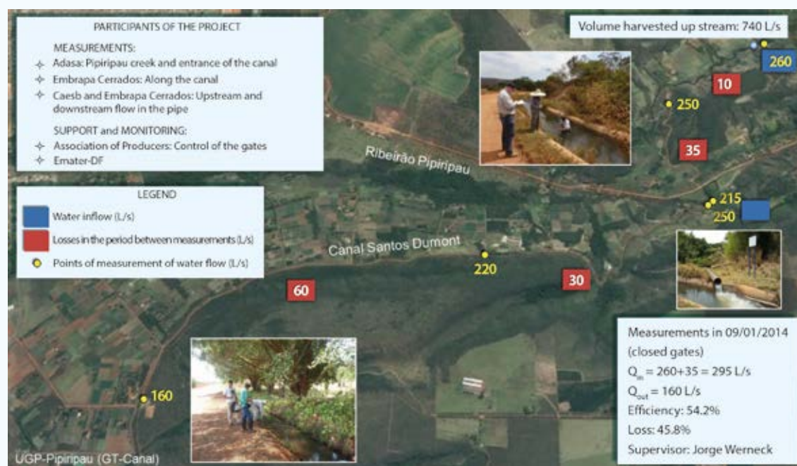
Figure 4. Photos and results of the joint campaign of inflow monitoring for determination of the losses along the main stretch of the Santos Dumont canal.
